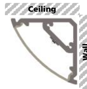
Version without switch (suitable for mounting in corner of wall/ceiling)
